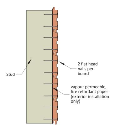
Face fixing Horizon - Stepped Profile (Installed horizontally)
