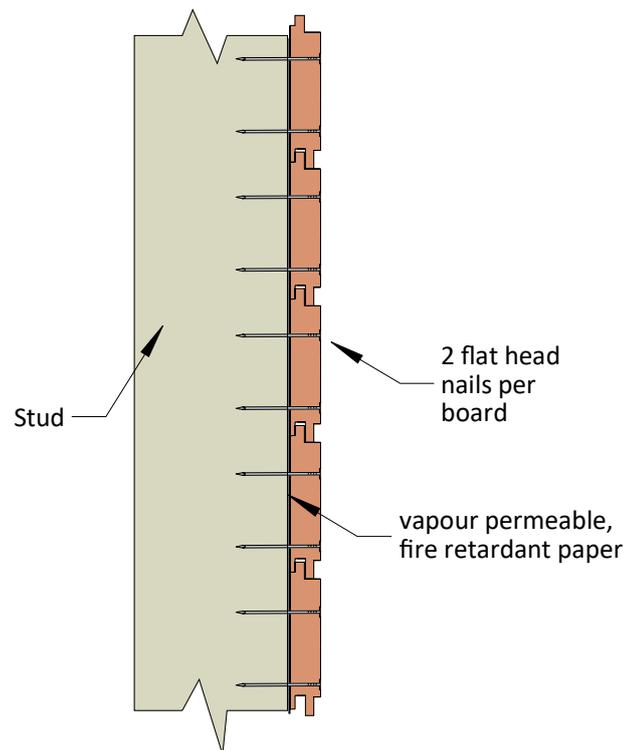
**Face Fixing External Cladding
