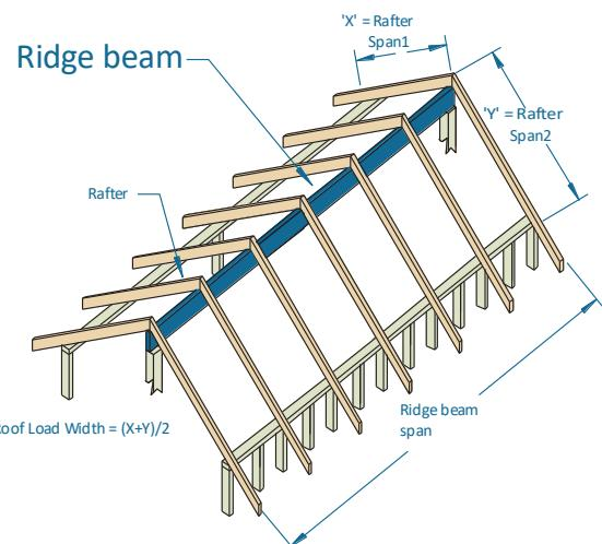
Enter single span table at 3000 roof load width with column and read down to span equal to or greater than 4500 mm
