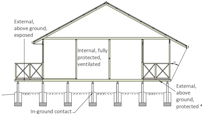
External timbers are regarded as protected in AS 1684 if they are covered by a roof projection (or similar) at 30° to the vertical and they are well detailed and maintained (painted and kept well ventilated).
