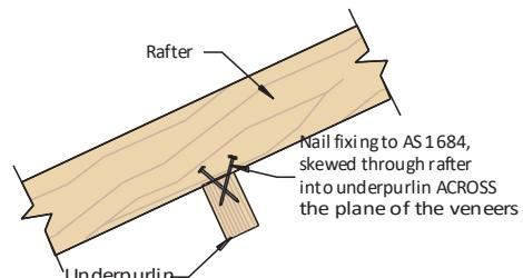
Rafters are NOT to be skew nailed to the underpurlin - with the nails parallel to the direction of the veneers
