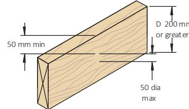
NOTE: Not more than 1 hole per 1800 mm of span
