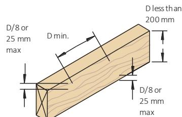
NOTE: Not more than 3 holes per 1800 mm of span
