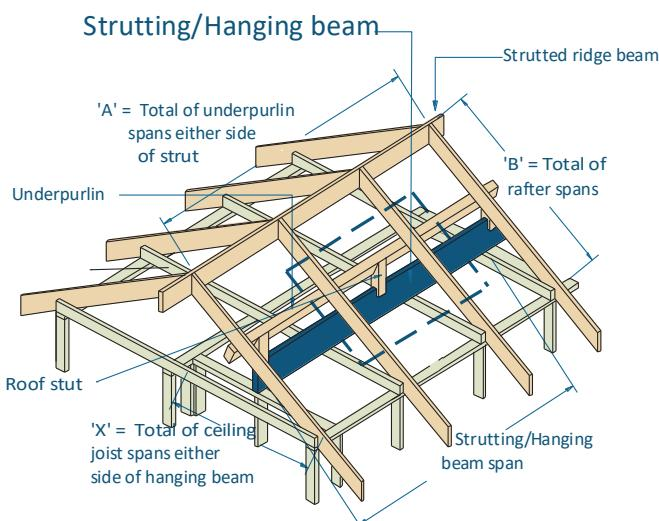
**Roof Area Supported = A/2 x B/2 Ceiling Load width = X/2**
