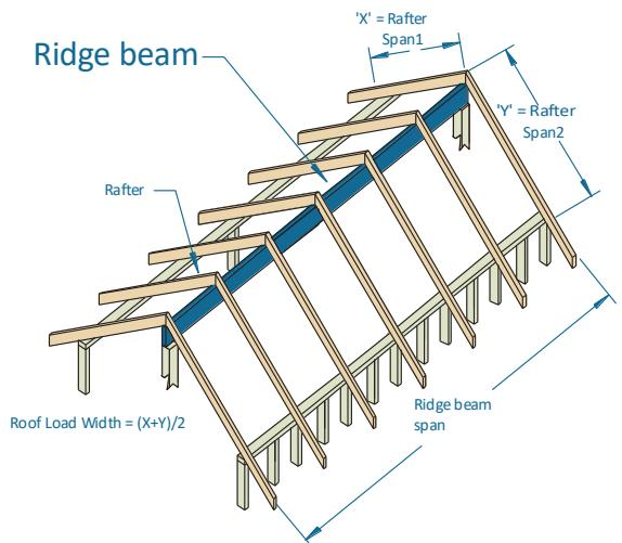
Enter single span table at 3000 roof load width with column
