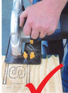
The sawing through the thickness to produce sections of a lesser thickness may decrease the integrity of the SmartLVL and is therefore NOT recommended under any circumstances.
