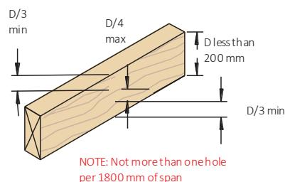
NOTE: Not more than one hole per 1800 mm of span
