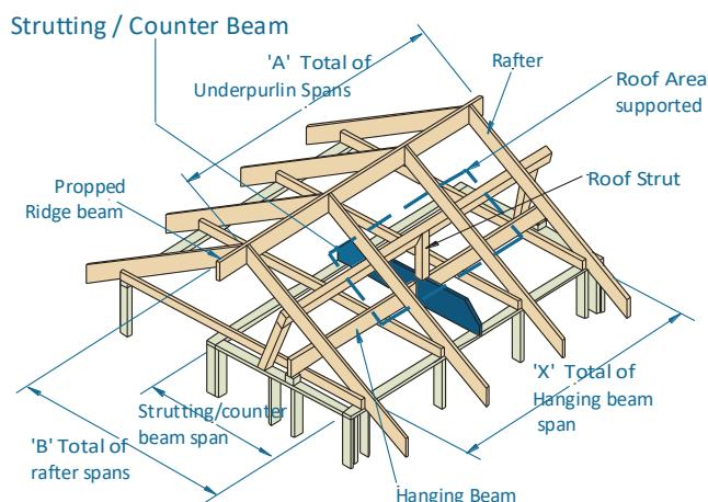
Roof Area supported = A/2xB/2 Counter/Strutting beam spacing = X/2
