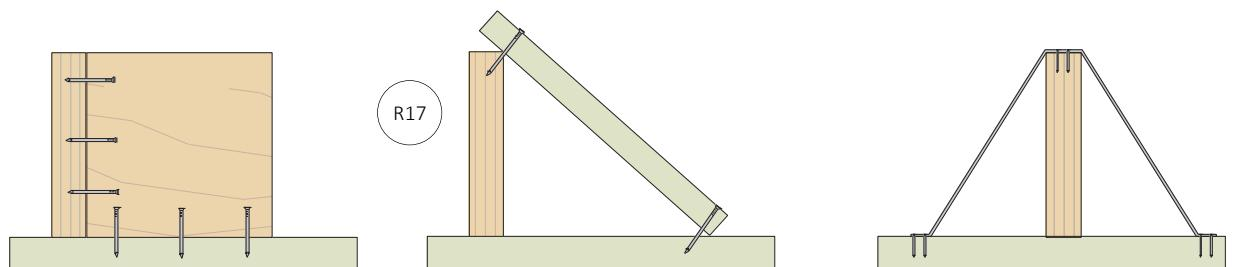
(a) Block skew nailed to beam and to support with 3/75 mm skew nails to each member.
