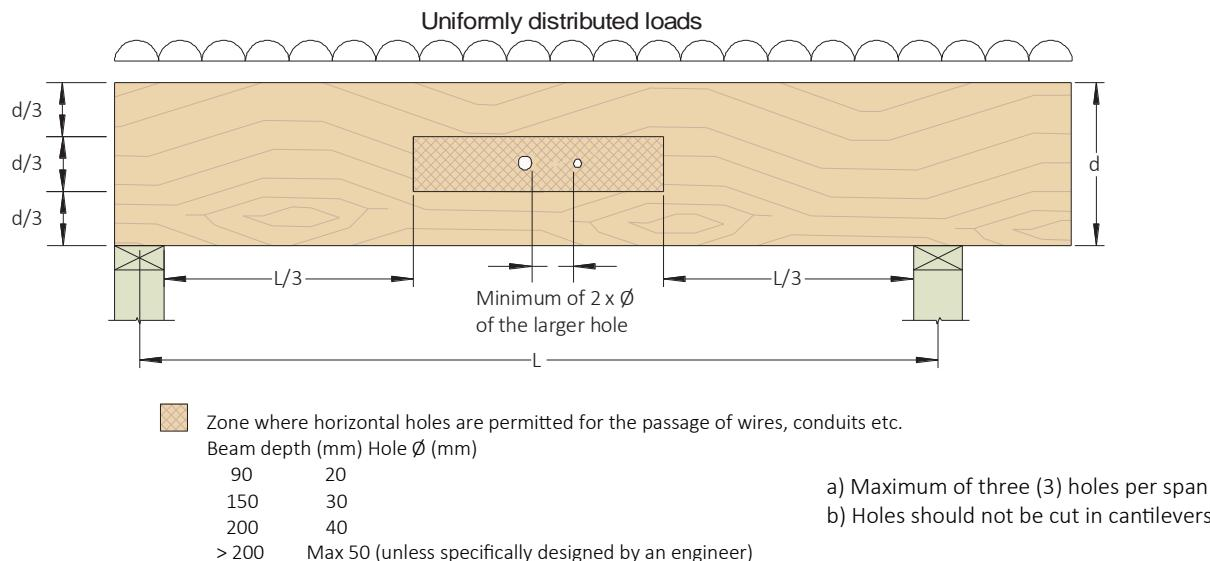
A 25 mm  $\phi$  or smaller hole may be cut at the middle  $\frac{1}{3}$  of the beam depth anywhere along the span, except for the area that is within 150 mm of clear distance between the face of the support and the nearest edge of the hole (see Figure 3 on next page), provided the following conditions are all met:
