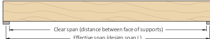
Diagram (b) shows beam where bearings at each end have been oversized. (This is frequently the case for beams that bear onto brickwork or concrete walls where the thickness of the wall is in excess of the area required to give the beam bearing capacity).
