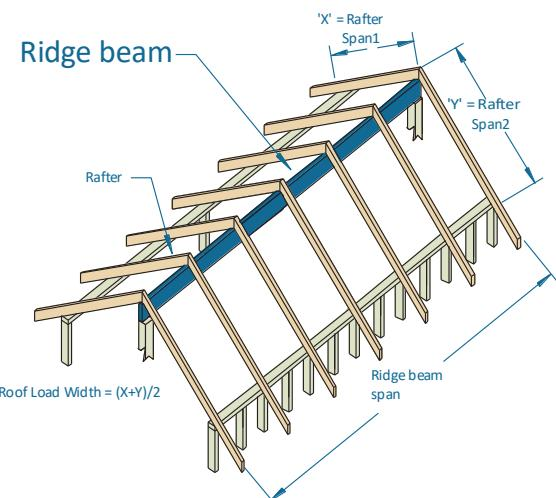
Enter single span table at 3000 roof load width with column and read down to span equal to or greater than 4500 mm in the 40 kg/m<sup>2</sup> row
