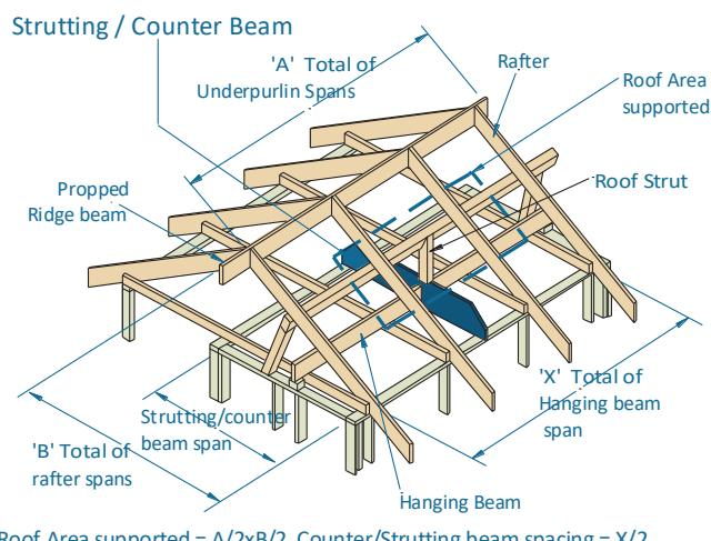
$$\text{Roof Area supported} = \frac{A}{2} \times \frac{B}{2} \quad \text{Counter/Strutting beam spacing} = \frac{X}{2}$$
